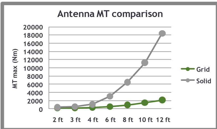
Similarly, Yagi antennas are subjected to significantly less horizontal loading and turning force than solid parabolic antennas:
