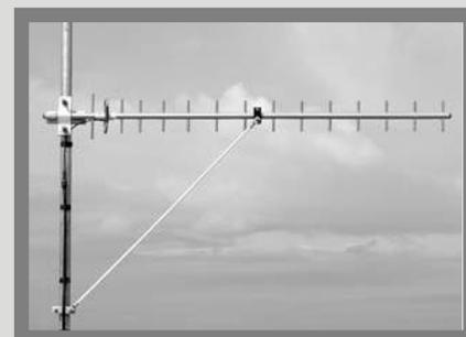
Typical lightweight Yagi antenna
