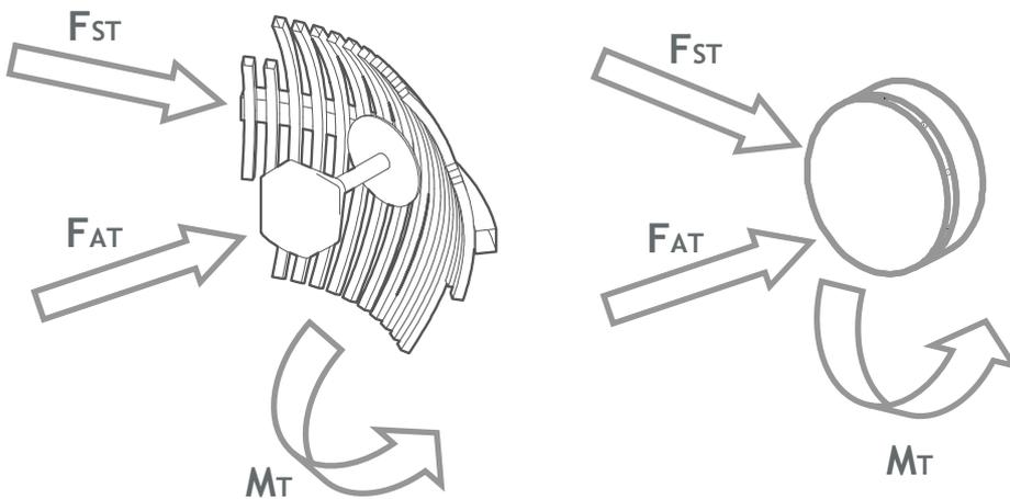
The table and graphs below compare the average frontal loading (FAT: Force Axial on mounting Tube), horizontal loading (FST: Force Sideways on mounting Tube) and turning forces (MT: Moment torque on mounting Tube) for parabolic grid antennas compared with solid parabolic antennas at a wind speed of 200 km per hour:
